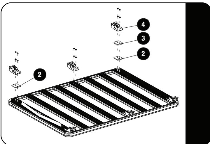
🔄 Loosely assemble the three Grab On Foot Sets (Item 4) onto the slats indicated in 2.2 as shown using M8 Flat Washers and M8 Nyloc Nuts.
