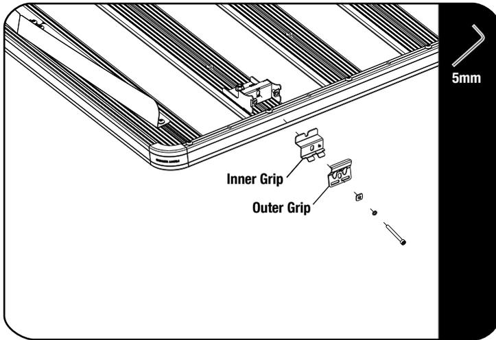
Loosley fit one Inner Grip and one Outer Grip to each Grab On Foot using a M5 Cap Screw, M6 Spring Washer and M6 Cap Screw Washer removed.
