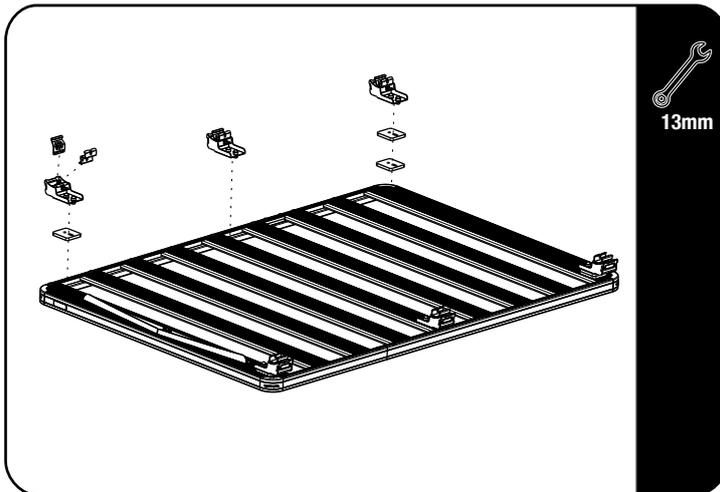
↻ Loosely assemble the two Grab On Foot Sets (Item 3) onto the slats indicated in 2.1 as shown using M8 Flat Washers and M8 Nyloc Nuts.
