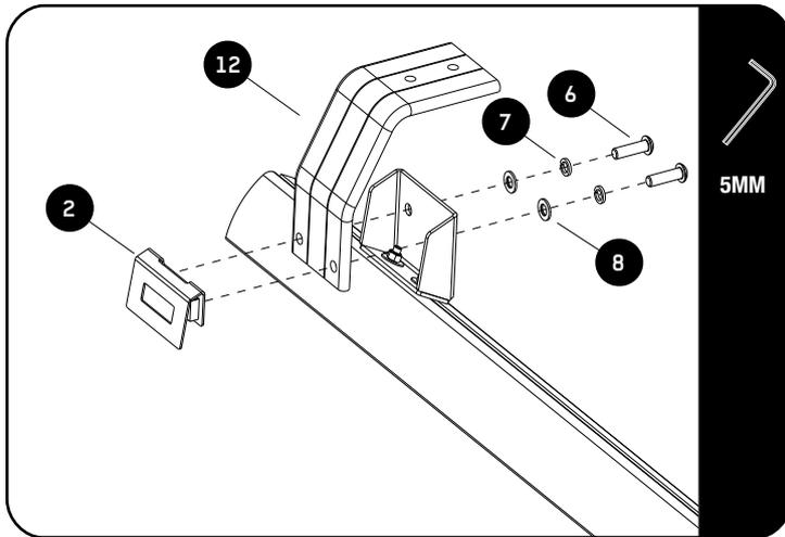
Assemble the Legs (Item 12) to the Leg Mount (Item 3) by using M8 x 20 Button Heads, M8 Spring Washers, M8 x 19 x 2SS Flat Washers (Items 6, 7 & 8) and the Nut Plates (Items 2).
