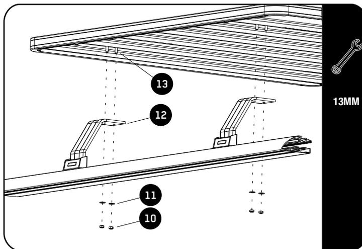
Loosely fit your Slimline II Rack by using M8 x 25 Hex Bolts, M8 x 16 x 1.6SS Flat Washers and M8 Nylocs (Items 10, 11, 13) as shown.
