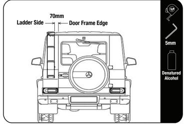
Swing open the Gutter Clamp. Fit the top assembly into vehicle's gutter and let the Bottom Support rest against the vehicle.
