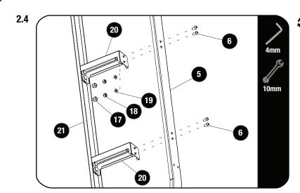
Assemble the two Ladder Rungs (Item 20) to the Ladder Side RH (Item 21) and then assemble Ladder Side LH (Item 5) as shown, using eight M6x12 Button Head Screws, eight M6 Flat Washers and eight M6 Nyloc Nuts (Item 6, 19 & 18). Finish off by placing eight M6 Nut Caps (Item 17) on the M6 Nyloc Nuts.
