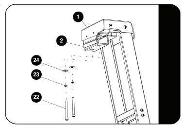
Loosely insert two M6x60 Cap Screws with two M6 Spring Washers and two M6x19x1SS Flat Washers (Item 22, 23 & 24) through the Gutter Clamp LH (Item 2) into the Ladder Top Clamp LH (Item 1) as shown.
