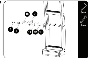
Assemble the Bump Stop (Item 9) to the Bump Stop Plate (Item 7) using the M5x16 Button Head Screw, one M5 Flat Washer and one M5 Nyloc Nut (Item 8, 11 & 12). Assemble the Bump Stop assembly to the right hand side (left hand side for RH installation) of the ladder using two M5x10 Button Head Screws, two M5 Flat Washers and two M5 Nyloc Nuts (Item 10, 11& 12). Finishing off placing three M5 Nut Caps (Item 13) on the M5 Nyloc Nuts.
