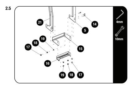
Assemble the Bottom Support (Item 15) and the Ladder Rung (Item 16) to the assembly in 2.4 using six M6x16 Button Head Screws, six M6 Flat Washers and six M6 Nyloc Nuts (Item 14, 19 & 18). Finish off by placing six M6 Nut Caps (Item 17) on the M6 Nyloc Nuts.
