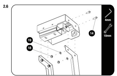
Assemble the Ladder Top in 2.3 to the assembly in 2.5 using four M6x16 Button Head Screw, four M6 Flat Washers and four M6 Nyloc Nuts (Item 14, 19 & 18)
