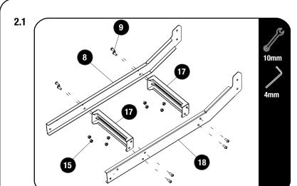
Secure the two Angled Ladder Rungs (Item 17) to the Top RH Ladder Side (Item 8) and the Top LH Ladder Side (Item 18) using eight M6x12 Button Head Screws and eight M6 Nyloc Nuts (Item 9 & 15). Finish off by placing M6 Nut Caps (Item 14) over the M6 Nyloc Nuts (Item 15).
