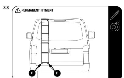
Apply masking tape to the door where the ladder is resting against the door.
