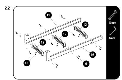
Secure the three Ladder Rungs (Item 12) to Bottom RH Ladder Side (Item 11) and Bottom LH Ladder Side (Item 16) using twelve M6 x 16 Button Head Screws and twelve M6 Nyloc Nuts (Item 9 & 16). Finish off by placing M6 Nut Caps (Item 14) over the M6 Nyloc Nuts (Item 15).
