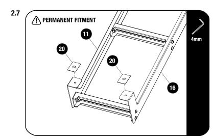
Remove the backing tape from the 45mm Rubber Strip (Item 20) and secure it to the bottom tabs on Bottom RH Ladder Side (Item 11) and Bottom LH Ladder Side (Item 16), aligning the hole in the 45mm Rubber Strip with the holes in both bottom tabs.
