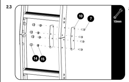
Secure the top assembly to the bottom assembly using four Ladder Joining Plates (Item 10), with eight M6x16 Button Head Screws, eight M6 Nyloc Nuts (Item 7 & 15). Finish off by placing M6 Nut Caps (Item 14) over the M6 Nyloc Nuts (Item 15).
