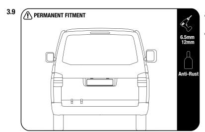
Using a 6.5mm drill bit, drill a pilot hole in the center of each of your markings. Open the holes using a 12mm drill bit.
