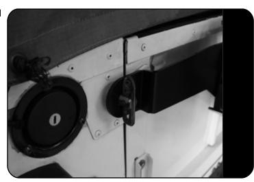
Close the Spare Wheel Carrier to ensure that it locates over the anti loose fastener.
