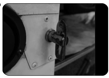
Remove both anti loose fasteners and add two M12 Flat Washers (Item 17) to space the anti loose fasteners away from the vehicles body.
