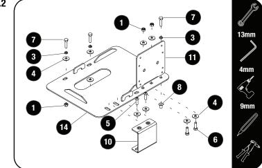
Fit the Battery Support Bracket (Item 10) under the windscreen wiper fluid bottle using the fasteners removed in 2.1.
