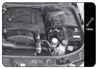
Bolt the charger onto the Mounting Bracket (Item 11). Position the battery on the Battery Bracket and fit the Battery Strap (Item 9).
