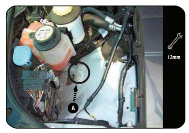
Relocate the alarm horn on the wheel arch towards the head light and reroute the wiring if necessary. Remove the mounting bolts (Item A) from the windscreen wiper fluid bottle as indicated in 2.1.
