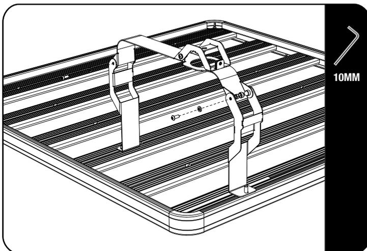
Assemble the Lockable Strap For The Water Cap to the upright brackets by placing it on the inside of the upright brackets. Use the fasteners that you removed in Step 2.2.
