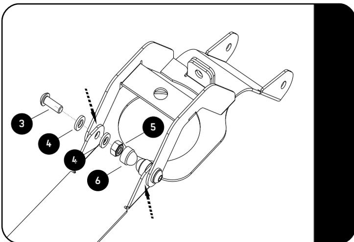
Assemble the Lockable Bracket (Item 2) to the Strap (Item 1) using M6 x 16 Button Head Bolts, M6 x 12 x 1SS Flat Washer and M6 Nyloc Nuts (Items 3, 4 & 5) as shown.
