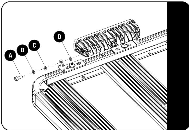
↻ Fit the LED light to the brackets as shown, using the fasteners supplied with the light.
