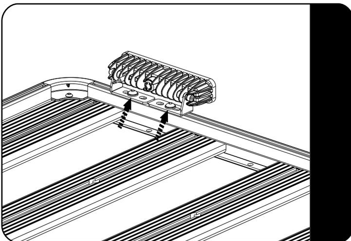
↻ Fully tighten the M8 Button Head Bolts fitted in 2.4.
