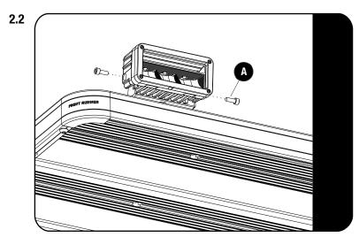
Fit the LED light to the bracket as shown, using the fasteners supplied with the light.
