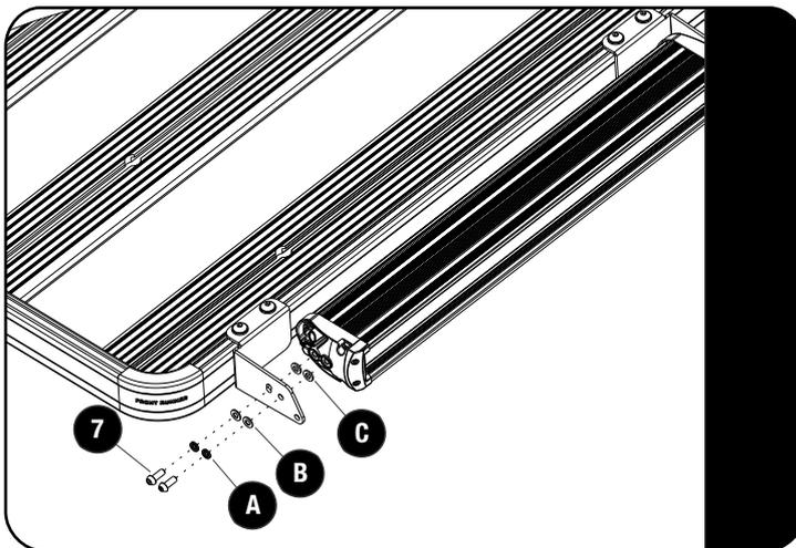
Fit the LED light to the brackets as shown, using the M6 x 16 Button Head Bolts (Item 7) and fasteners supplied with the light .
