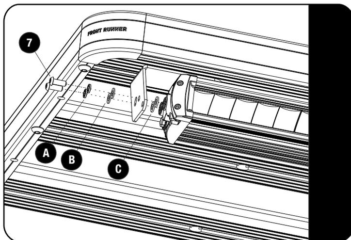
Fit the LED light to the brackets as shown, using the M6 x 16 Button Head Bolts (Item 7) and fasteners supplied with the light .
