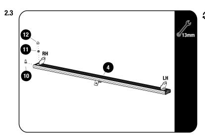
Fit the Light Bar Bracket 01 LH / RH (Item 4) for for Front Runner 40" Light Bar, using M8x16 Hex Bolt & M8 Nyloc Nut (Items 10 & 11). Fit the Light Bar and center on slat before fully tightening the brackets.
