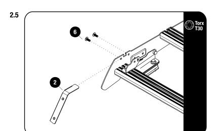
Secure the Wind Fairing Side Supports LH / RH (Item 2) to the foot rails top holes as shown using M6x16 Flange Button Head (Item 6).
