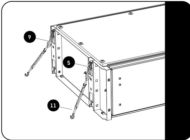
🔄 Connect the C-hooks (item 9) onto the D-rings (item 5) on the drawers upright. Connect the turnbuckles (item 11) on the other side of the C-hooks and hook it into the tie-down that are fitted to the vehicle.
