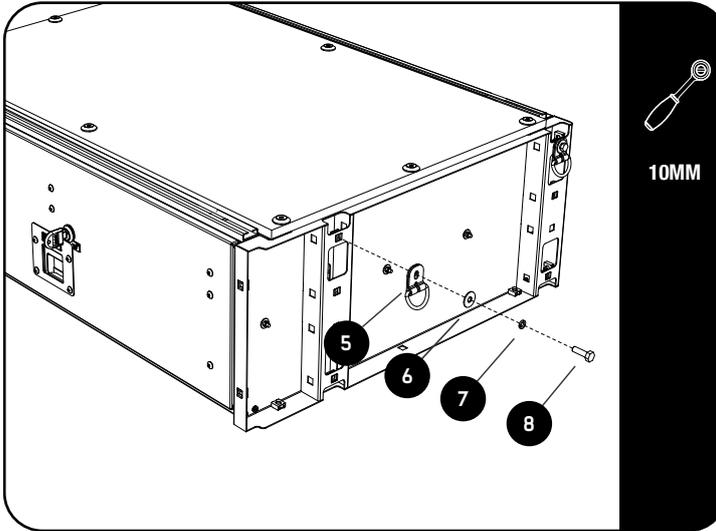
Secure the 4 D-Rings (item 5) on both sides of the drawer using the fasteners shown.
