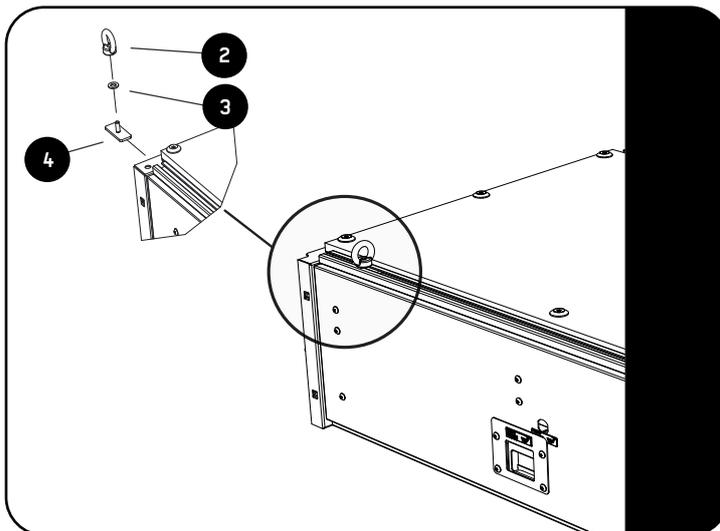
🔄 Assemble the eye-nuts (item 2) with a M6 nylon washer (item 3) and a stud plate (item 4) and slide them into place.
