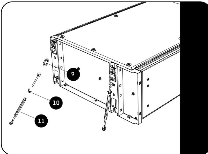
Assemble each of the 4 turnbuckles (item 12) with a wing nut (item 10) as shown. The wing nut will be used to lock the turnbuckles after they have been set.
