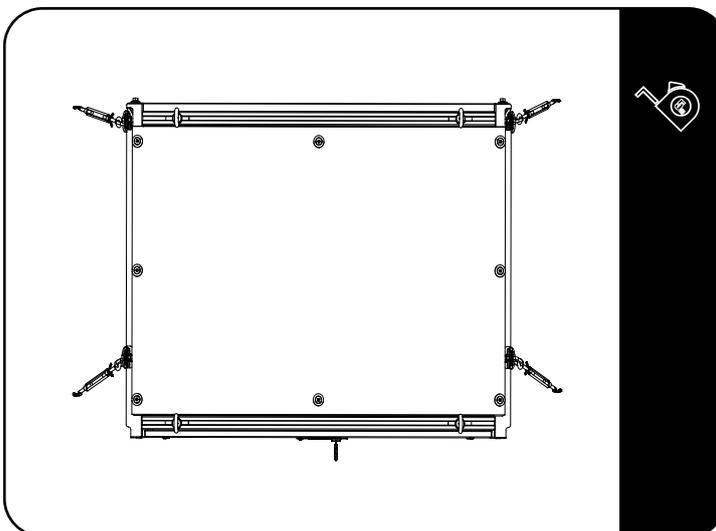
Place the drawer in the vehicle and position as desired. Making sure the turnbuckles are pulling outward to prevent the drawer from moving after it has been secured.
