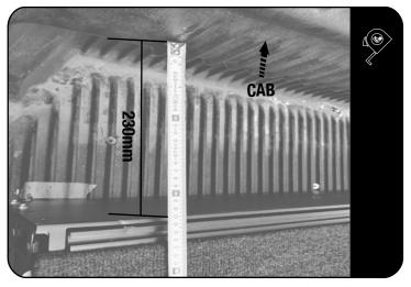
Position the drawer 230mm from the back of the cab as shown.
