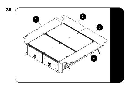
Place the relevant deck sets in place as shown, making sure that you slide it into the C-clip of the Side Wings.
