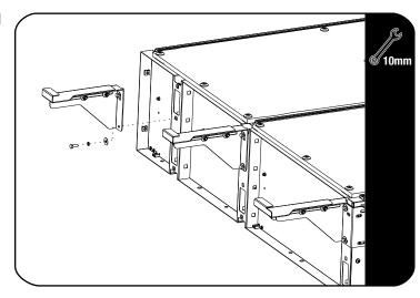
Secure the three LH / RH Side Wings (SSWS001) to the drawer system, using M6x20 Hex Bolts, M6 Spring Washers & M6x19 Flat Washers.
