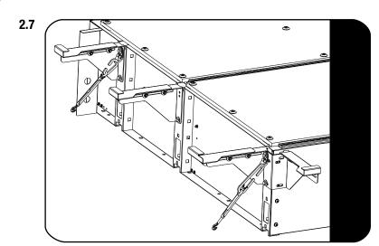
Secure the Drawer System in position using the Turnbuckles (supplied with SSDR010) and Carabiner (Item 9) as shown.
