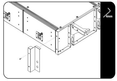
Secure the two Face Plates LH / RH (Item 5 & 6) to the drawer using four M6x12 Button Head Screws (Item 12).
