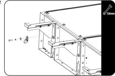
Secure the D-Rings, using the fasteners supplied with the drawer system (SSDR010) as shown. Two on the right and two on the left hand side.
