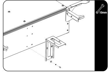
Secure the Rear Wing Sets as shown, using M6x20 Hex Bolts, M6 Spring Washers & M6x19 Flat Washers.
