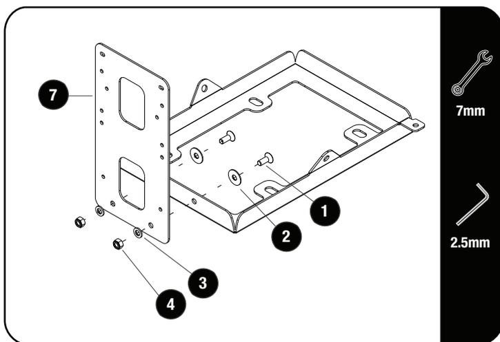
☺ Using two M6 x16 Countersink Screws, two M6 x 19 x 1SS Flat Washers, two M6 x 12 x 1SS Flat Washers and two M6 Nyloc Nuts (Items 1, 2, 3 & 4) fasten the Battery Device Mounting Plate (Item 7) to the Battery Bracket.
