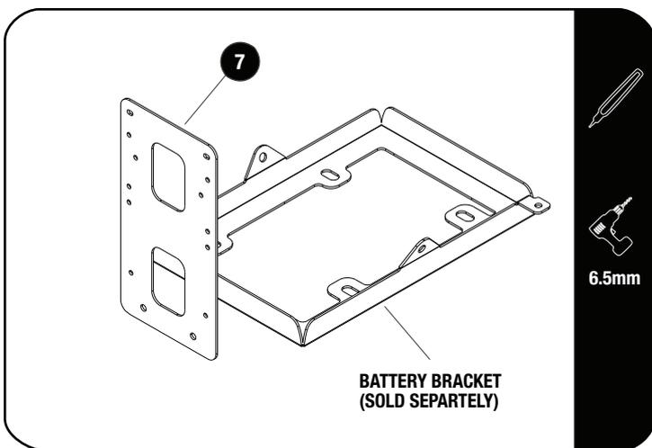
☺ Determine where on the Battery Bracket you would like to mount the Battery Device Mounting Plate (Item 7). Using a marker pen, mark the two holes.
