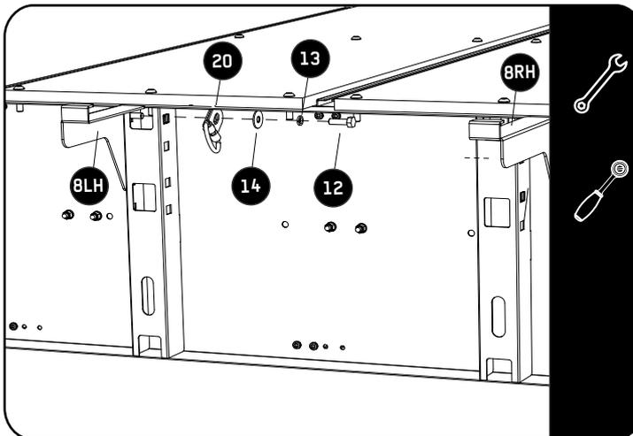
Refer to 1.1 for wing placement. Fit item 20 to the rear left and rear right side of the drawer as shown.
