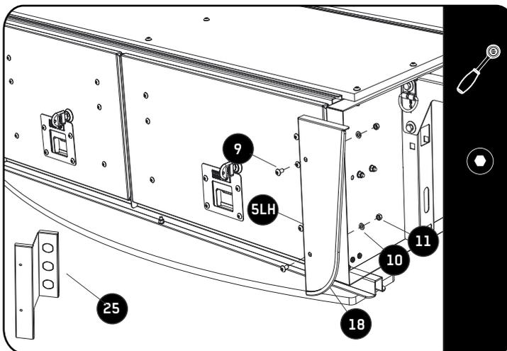
Secure the Front Faces (Item 18 or 25) to the drawer using M5 x 12 Button Heads, M5 Flat Washers and M5 Nyloc Nuts (Items 9, 10 & 11) as shown.
