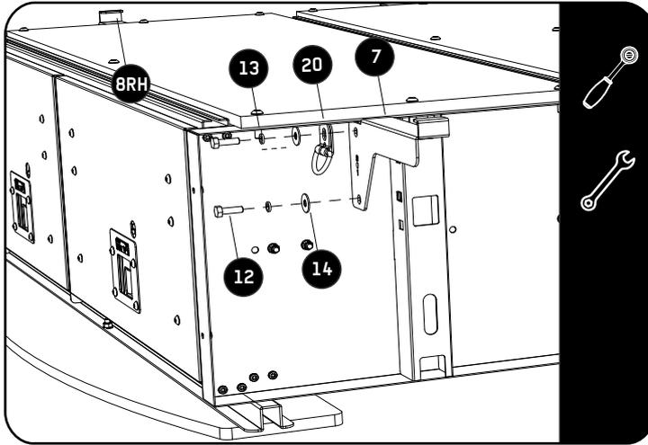
Place the drawer in the vehicle before assembling the wings onto the drawer. Refer to 1.1 for wing placement. Fit item 20 to the front left and the front right side of the drawer as shown.
