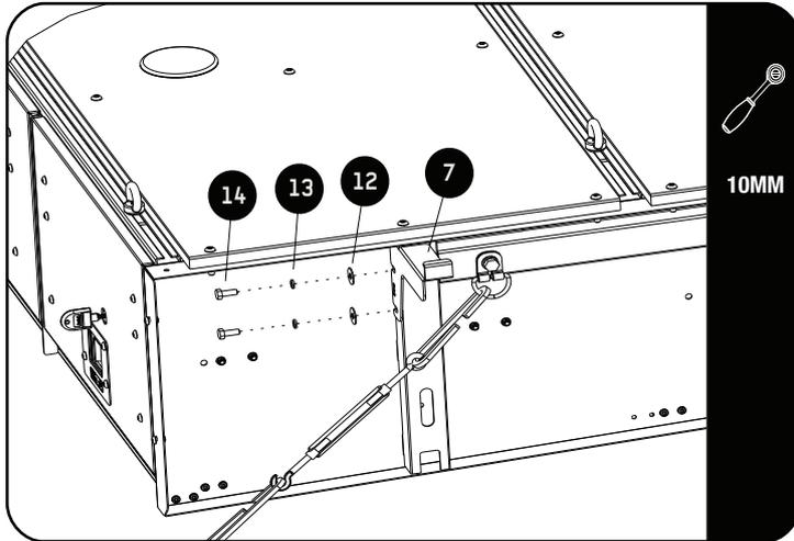
Secure the Side Wings (Items 4, 5, 6 & 7) using M6 x 16 Hex Bolt, M6 Spring Washers and M6 x 19 x 1SS Flat Washers (Item 12, 13 & 14) as shown.
