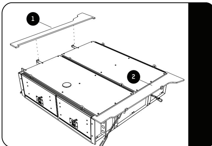
Place the Side Decks (Item 1 & 2) onto the Drawer making sure that you slide it into the C-clip of the Front and Rear Side Wings.
