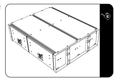
Place the drawer system into the vehicle, locating it as far back as possible without interfering with the rear door operation.
