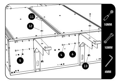
Fit the four mounting brackets, two left and two right. There are two different height options available when mounting the brackets. Choose the option best suited to your vehicle.
