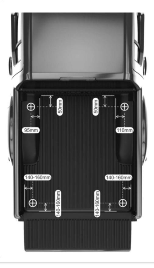
( H ) Using the components received with SSDS501, secure the four D-ring's (Item 31) to the inside of the Load Bay. You will be bolting through each of the holes drilled in Step 2G using a M6 x 25 Hex Bolt, two M6 x 19 Flat Washers and a M6 Nyloc Nut per D-ring (Items 32, 33, 34) as shown.
