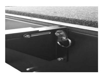
( **I** ) Remove the four tie down hooks from the vehicle's loadbay.
