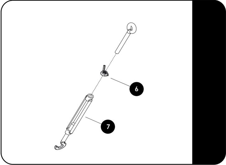
Assemble each of the 4 Turnbuckles (Item 7) with a Wing Nut (Item 6) as shown. The wing nut will be used to lock the Turnbuckles after they have been set.
