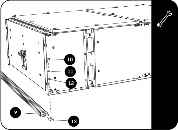
Slide 2 channel nuts into the track. Center the track under the drawer and secure with the fasteners that are shown.
