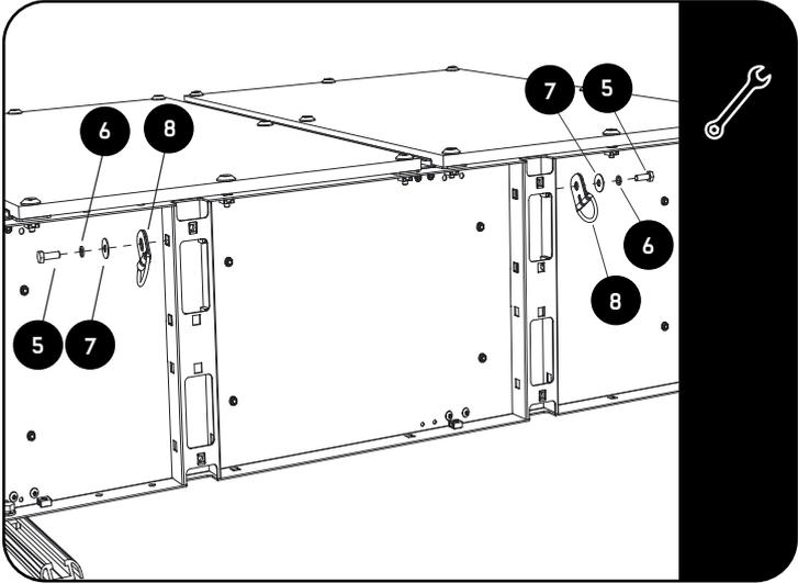
Secure the 4 D-Rings on both sides of the drawer as shown.
