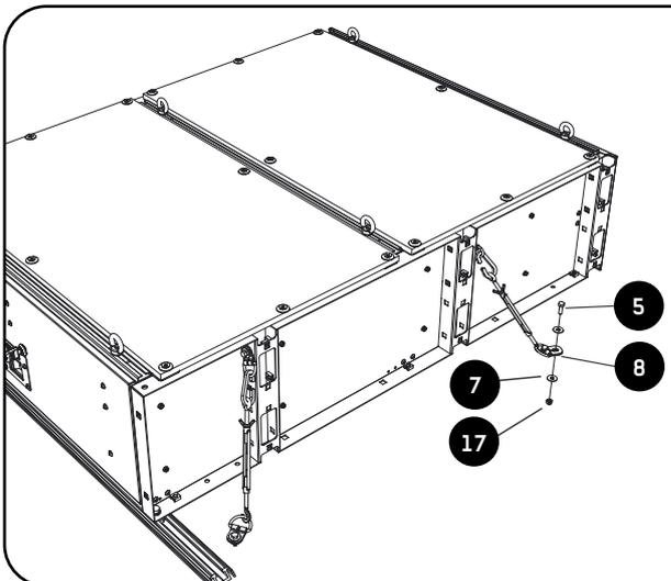
Use the fasteners that are shown to secure the drawer to the vehicle.
