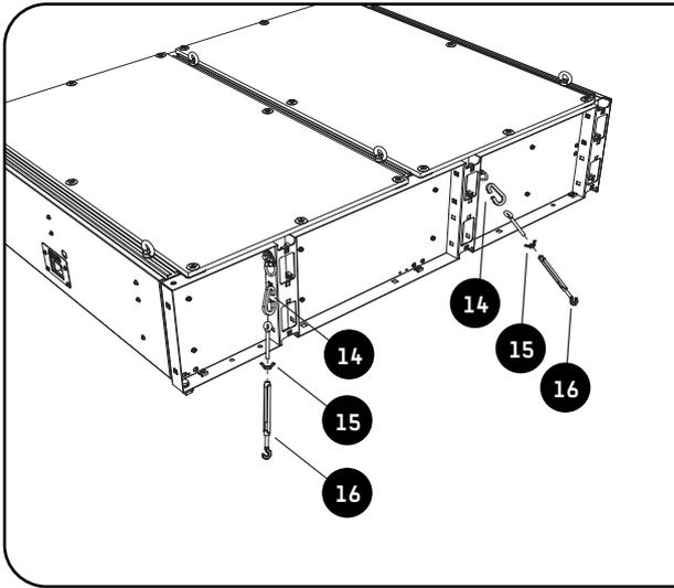
Assemble each of the 4 turnbuckles with item 15 as shown. Item 15 will be used to lock the turnbuckles after they have been set.
