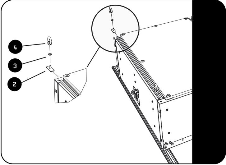
Assemble the 6 eye-nuts and slide into place.
