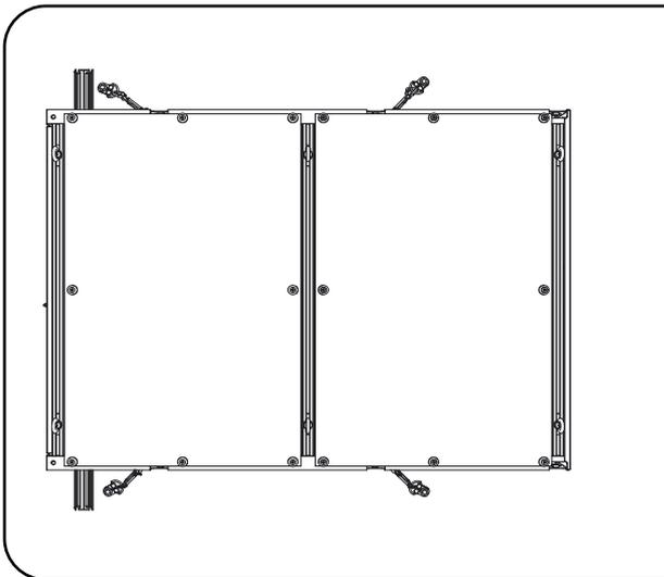
Place the drawer into the vehicle and position as desired. Making sure the turnbuckles are pulling outward to prevent the drawer from moving after it has been secured. Mark and drill 6.5mm holes using the D-rings as a guide.
