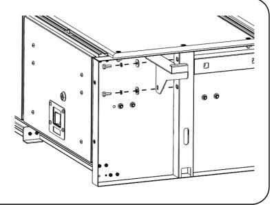
(E) Secure the Left and Right Rear Wings (Item 11) to the Wing Brackets fitted in Step 2F using four M5 x 12 Button Head Bolts, four M5 Flat Washers and four M5 Nyloc Nuts (Items 23, 24, 25) as shown.
