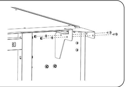
( **F** ) Secure the Left and Right Front Faces (Item 10) to the Drawer System using four M5 x 12 Button Head Bolts, four M5 Flat Washers and four M5 Nyloc Nuts (Items 23, 24, 25) as shown.
