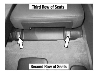
( **B** ) Secure the left and right hand Mounting Brackets (Item 14) to the vehicle as shown below, using the original bolts removed in Step 2A.
