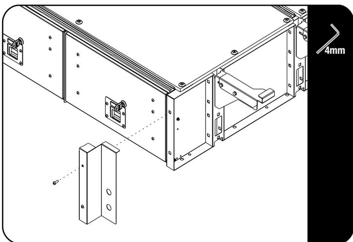
Secure the two Face Plates LH / RH (Item 5 & 6) to the drawer using four M6x12 Button Head Screws (Item 12).
