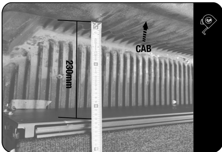
Position the drawer 230mm from the back of the cab as shown.
