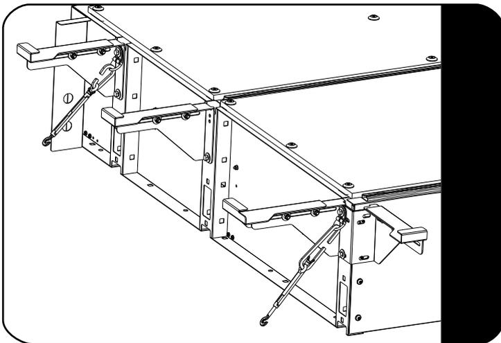
Secure the Drawer System in position using the Turnbuckles (supplied with SSDR010) and Carabiner (Item 9) as shown.
