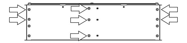
(F) Using six M6 x 16 Hex Hex Bolts, six M6 Spring Washers and six M6 x 19 Flat Washers removed in Step 2E, secure the Rear Support (Item 23) to the back of the Drawer System as shown.
