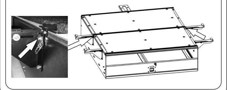
Position the Corner Wing Assemblies from Step 2B over the corners of the Drawer as shown. Secure the Assemblies to the Drawer using the remaining M6 x 20 Hex Bolts, M6 x 19 Flat Washers and M6 Spring Washers. As in Step 3B, secure a D-Ring (Item 4) to each of the rear corners as shown.
