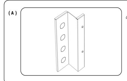
Twist the pre cut knock outs to remove. These cut outs can then be used to fit Front Runners range of electrical panel inserts.
