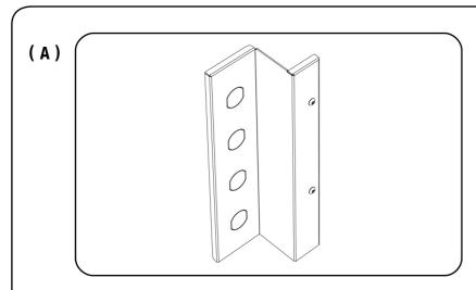
Twist the pre cut knock outs to remove. These cut outs can then be used to fit Front Runners range of electrical panel inserts.
