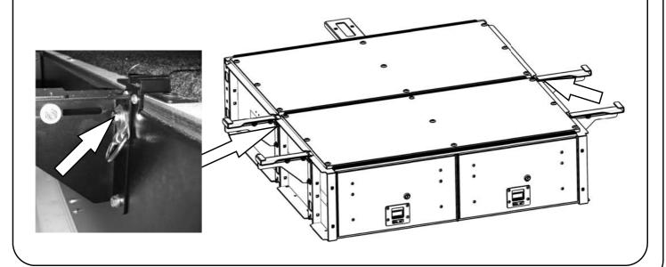
Position the Rear Corner Assemblies from Step 2B over corners of the Draw as shown. Secure the Assemblies to the Drawer using four M6 x 20 Hex Bolts, four M6 x 19 Flat Washers and four M6 Spring Washers (Items 20, 21, 22) received with SSWS001 and the remaining fasteners from Step 2E. As in Step 3B, secure a D-Ring (Item 4) to each of the rear corners as shown.
