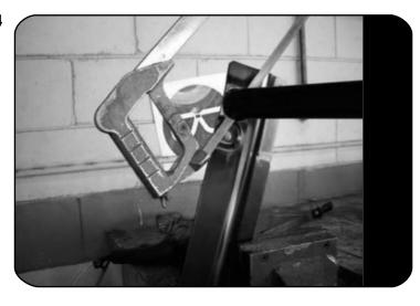
The safety support bracket must be modified. Clamp the 'flat' portion in a vice. Using your hack saw, cut the tube off as close to the plate as possible.
