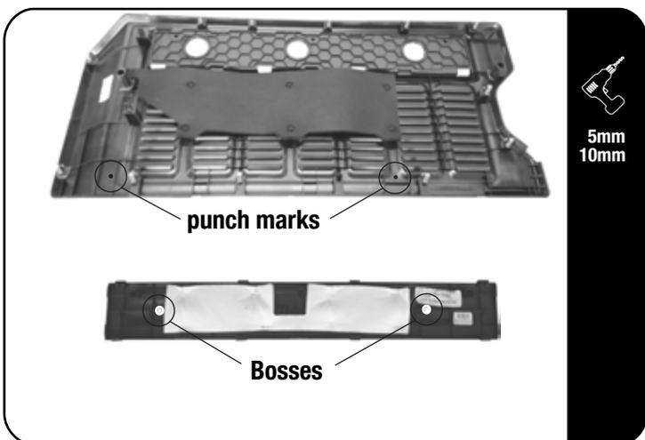
↻ At the inside of the trim panel, locate the two factory indicator punch marks.
