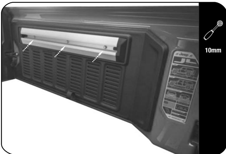
↻ If your vehicle has the cargo Rail fitted, remove it by loosening and removing the three bolts shown.
