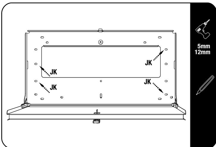
⌛ Drill 5mm pilot holes on the marks made, using light pressure and taking care only to drill through the interior panel. Widen the holes to 12mm.
