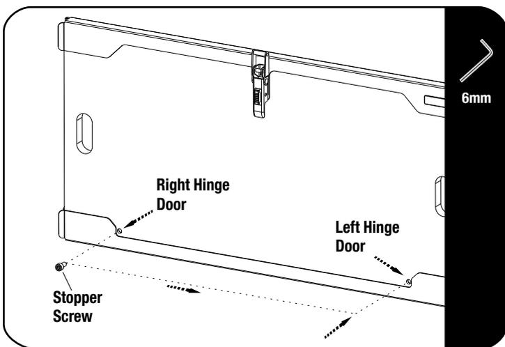
⌛ If your vehicle has a door that opens to the left side, you need to reposition the Stopper Screw. Do this by removing it from the left side of the Sliding Board and refitting it on the right side as shown in 2.1.
