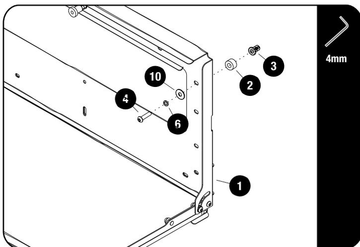
Secure the Drop Down Table using M6 x 25 Button Heads, M6 Spring Washers, M6 x 12 x 1 Flat Washers and Spacers (Items 2, 4, 6 & 10) as shown.
