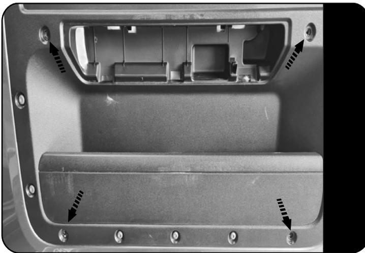
🔄 Remove the OEM Bolts as shown.
