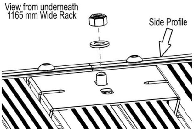
**All other Widths:** Push the Inter-slat Bracket against the inside of the Side Profile. Line up the best suited slot in the Inter-slat Bracket with the hole and Nyloc Nut at the end of the Additional Slat. Secure the Additional Slat to the Inter-slat Bracket using a M8 x25 Button Head Bolt and M8 Flat Washer (Items 5 &6). Tighten all bolts.
