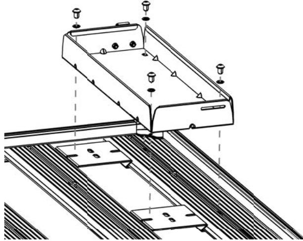
Tighten the four M8 Nyloc Nuts securing the Inter-slat Brackets to the Rack.
