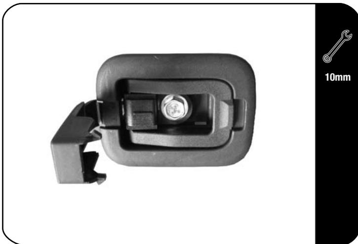
Loosen and remove the two tie down points located on the floor of the vehicle behind the rear passenger seats.
