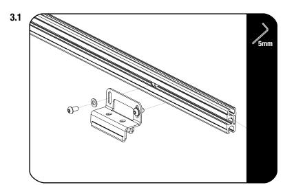
Loosely assemble the FPCR Feet (Item 7) using M8 x 16 Button Head Bolts, M8 Flat Washers and M8 Nyloc Nuts and slide them into the side profiles. They must still be able to slide freely.
