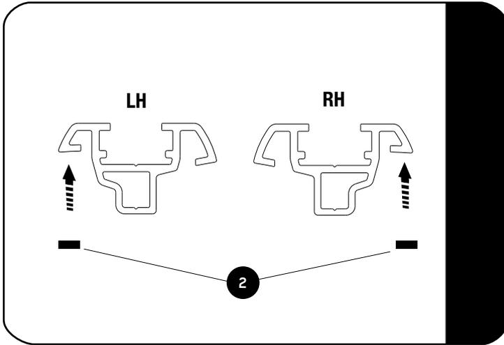
Fit the Foam Strips (Item 2) by removing the backing tape and apply them to the outside profile edge of each of the Tracks as shown in 2.3.
