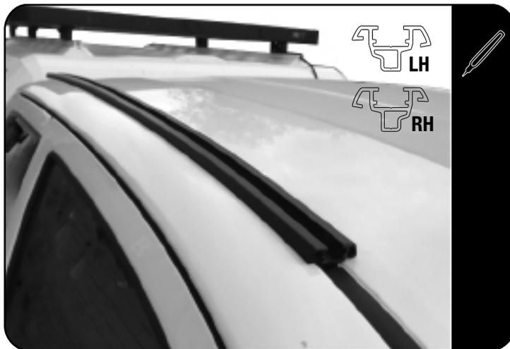
Place the LH Track into the LH ditch and RH Track into the RH ditch. Ensuring they are fully seated.
