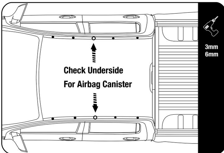
After marking the hole positions, check the underside for the airbag canister position. Some models have the canister positioned in the centre of the track.
