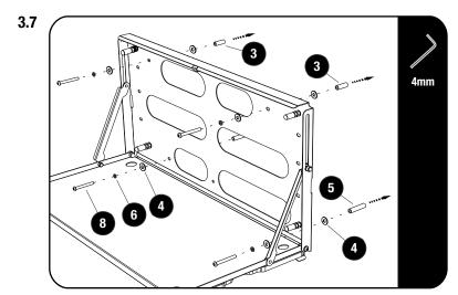
Insert two 30mm Spacers (Item 3) in the top two holes and two 35mm Spacers in the bottom holes drilled earleir in Step 3.5 and 3.6.
