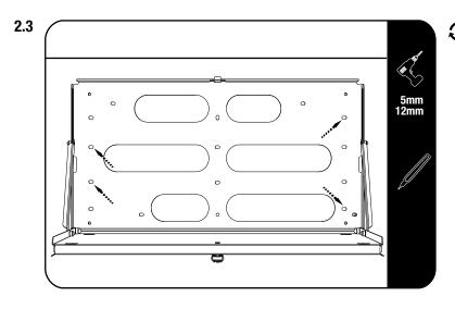
Open the table and mark out the four fixing points shown in 2.3.
