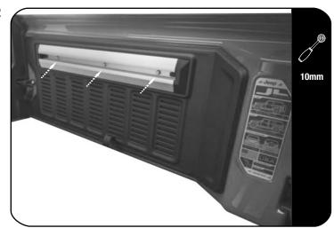
If your vehicle has the Sports Rail fitted, remove it by loosening and removing the 3 bolts shown.
