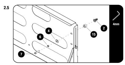
Secure the Drop Down Table using M6 x 25 Button Heads, M6 SS Spring Washer, M6 x 12 x 1 SS Flat Washers and Spacers (Items 4, 6, 7 & 15) as shown.
