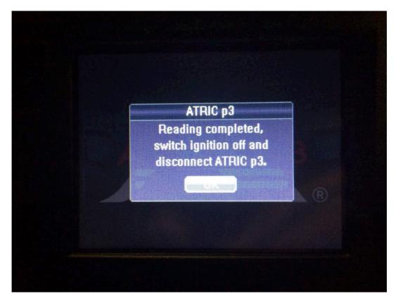
**Step 6** – Connect the Atric device to your computer and load the Atric P3 Software. Use the software to extract the file from the device and once this is done email it to sales@performancelandies.com with details of how you would like the map setting up and a list of all your current modifications.
