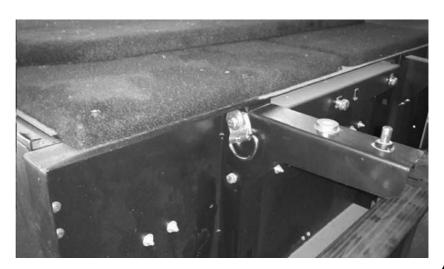
Secure the Draw System to the vehicle using the D-rings on the side of the Draw and the vehicle's mounting rings (Two in the front From Step 1A and two found behind the passenger seats). For each of the FRONT mountings use a Carabiner or small C-hook, a large C-hook and a Turn Buckle. For each of the REAR mountings use two large C-hooks and a Turn Buckle
