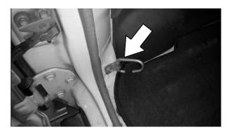
( **B** ) Looking at the sides of the Draw System, loosen and remove the rear D-ring as indicated by the arrow.
