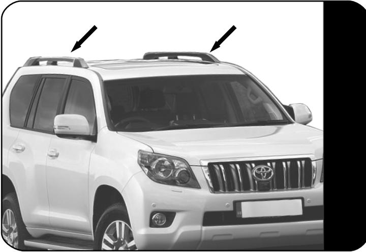
Remove the OEM rails from the left and right side of the vehicle.
