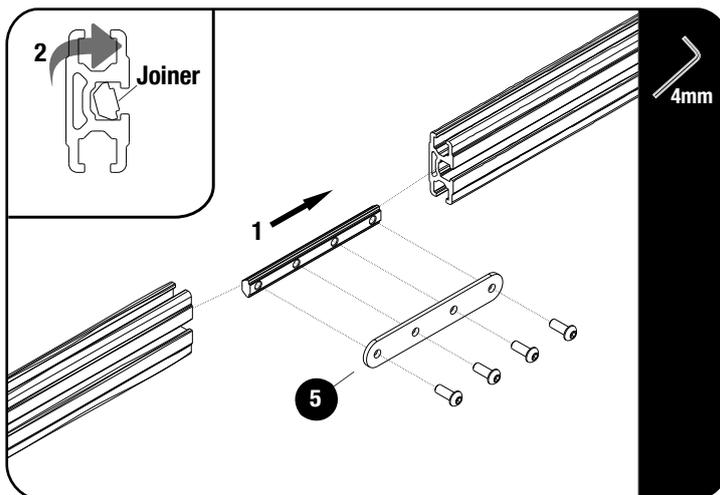
Place Joiner into the Side Profile and twist into position as shown. Refer to Item 4 on Page 4. Assemble the Side Profiles (Items 1 & 2) using the Rack Joiners (Item 5) and M6 x 16 Button Head Bolts and fully tighten. See 2.3 for Side Profile orientation.
