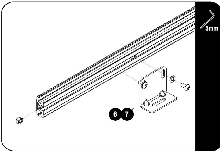
Loosely assemble the Feet (Item 7) using M8 x 16 Button Head Bolts, M8 Flat Washers and M8 Nyloc Nuts and slide them into the side profiles. They must still slide freely. Refer to Item 7 on page 4 for assembly. See 2.3 for positioning around Joiners
