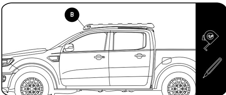
Place the foot rail on the vehicle's roof lining up the front slot center with the mark you made earlier and mark the centre of the remaining three slots.
