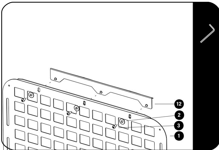
Loosley fasten the Curtain Airbag Mounting Bracket (Item 12) to the Molle Panel (Item 1) using three M6 x 16mm Button Head Bolts (Item 3) and Three M6 x 19 x 1 Flat Washers (Item 2) as shown in Figure 2.1.
