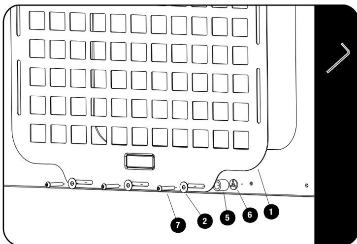
There are five round plastic caps under the rear window, remove the three middle caps. Loosley mount the bottom of the Molle Panel to the three mounting points under the rear window using M6 x 35mm Button Head Bolts (Item 7), M6 Flat Washers (Item 2), 20mm Spacers (Item 5) and M6 Plastic Retaining Washers (Item 6).
