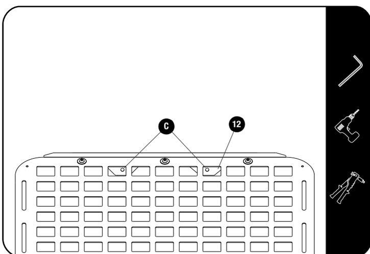
Push the Curtain Airbag Mounting Bracket (Item 12) upwards until it sits flush against the top window sill. Mark the location of the holes on the sill as seen in Detail C.
