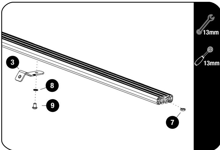
Slide one M8 Thin Nut (Item 7) into the T-Slot of the front slat. Center the Mid Support Bracket (Item 3) in the Middle of the slat and secure using a Schnorr Washer and M8 x 12 Button Head Bolt (Item 8 & 9). Fully tighten.
