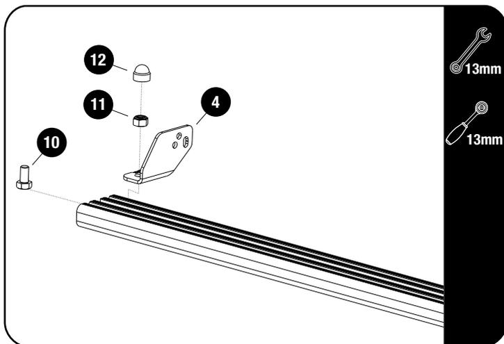
Fit the Light Bar Bracket 01 LH / RH (Item 4) for the 40" Light Bar, using M8 x 16 Hex Bolt & M8 Nyloc Nut (Items 10 & 11). Fit the light bar and center it on the slat before fully tightening the brackets.
