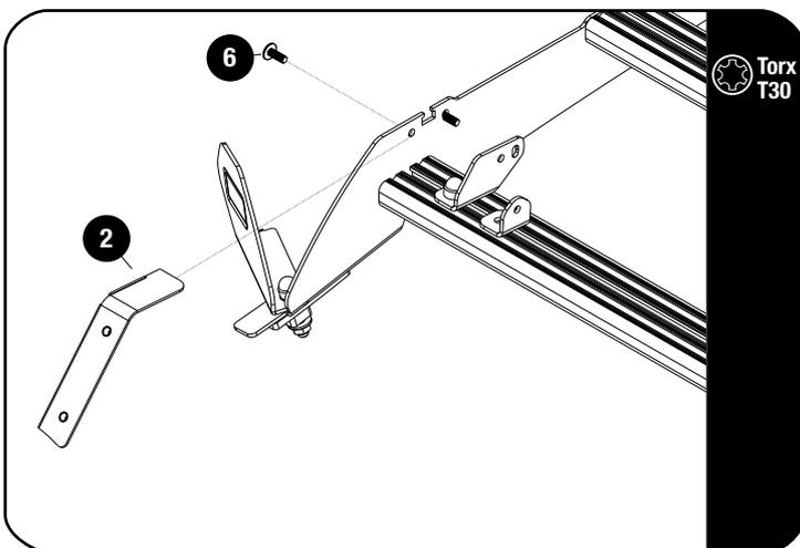
🔄 Swing over the Dimple plate to allow access to tighten the bolts.
