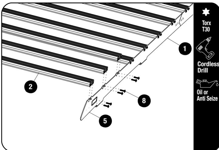
Assemble the 13 SlimSport Slats (Item 2) to assembly 2.1 using M6 x 25 Thread Forming Screws (Item 8).
