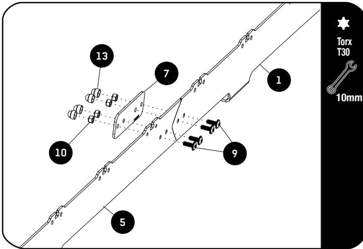
Assemble the Front and Rear Foot Rail (Items 1 & 5) with the Joiner Plate (Item 7) using M6 x 16 Flange Button Head Bolts and M6 Nyloc Nuts (Items 9 & 10) as shown.
