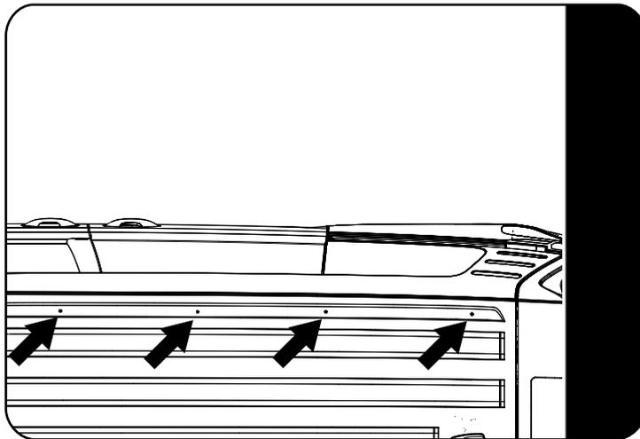
Remove the 8 Factory Fitted Caps on the roof.
