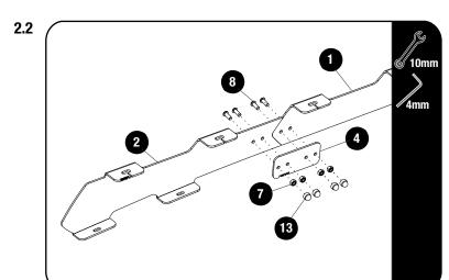
Assemble the Front and Rear Foot Rails (Item 1 & 2) together using the M6 x 16 Button Head Screws, Joiner plate and M6 Nyloc Nuts (Item 7,8 & 4).
