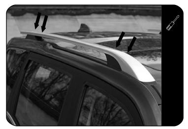
Start by removing the Factory OEM roof rails by uncliping the front and rear covers on the Rails.
