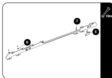
Place the Foot Rail over the M6 studs Protruding from the roof.
