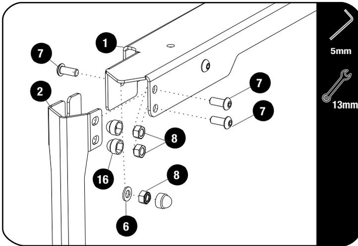
Assemble The Bottom Side Rails (Item 1) to the Front and Rear Legs (Item 2) as shown using the M8 x 12 Button Head Bolts M8 Nyloc Nut and M8 Nut Cap (Item 6,7 & 8).
