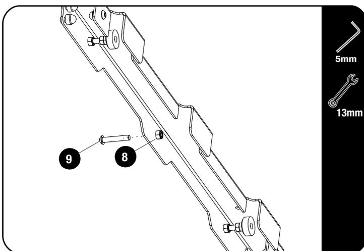
Secure three M8 x 50 Hex Bolts (Item 9) to each Side Rail (Item 1) using M8 Nyloc Nuts (Item 8) as shown.
