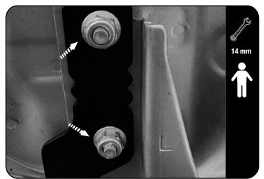
Position and align the bracket over the factory holes.
