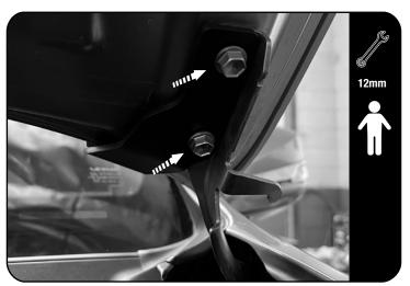
Position and align the bracket over the factory holes.
