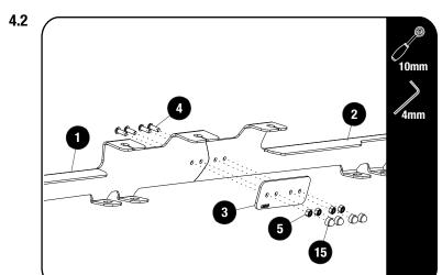
Assemble the Front and Rear Foot Rails (Items 1 & 2) using the Joiner Plate (Item 3) and M6 x 12 Button Head Bots and M6 Nyloc Nuts (Items 4 & 5) as shown.
