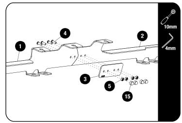
Assemble the Front and Rear Foot Rails (Items 1 & 2) using the Joiner Plate (Item 3) and M6 x 12 Button Head Bots and M6 Nyloc Nuts (Items 4 & 5) as shown.
