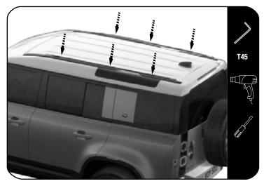
Remove the OEM rails from left and right side of the vehicle. It is advised to use a heat gun to heat the fasteners a little to soften the factory loc tite before removing.
