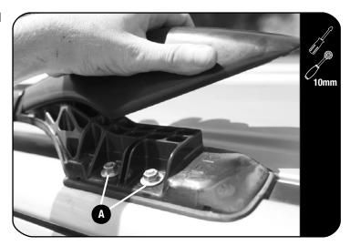
Starting at the front of the windscreen as shown, use a suitable panel tool to remove the OEM Roof Rail Cover.
