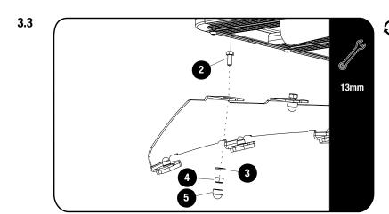
Fit your roof rack to the Foot Rails using M8 x 20 Hex Bolts, M8 x 16 x 1.6 Flat Washers and M8 Nyloc Nuts (Items 2, 3 & 4) as shown.
