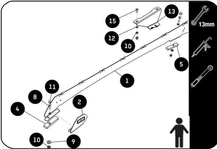
Apply a bead of sealant on the threads of the M8 x 40 Hex Bolts and secure the Foot Rail (Item 1) together with the Support Bracket (Item 13) and the Front and Rear Spacers (Item 4 & 5) to the Roof using M8 x 45 Hex Head Bolts, M8 x 19 x 2 Flat Washers and M8 Nyloc Nuts (Items 8,9 & 10).
