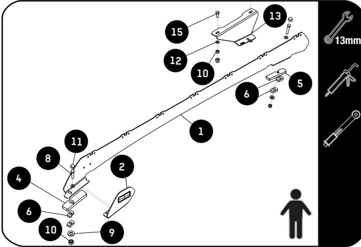
Apply a bead of sealant on the threads of the M8 x 40 Hex Bolts and secure the Foot Rail (Item 1) together with the Support Bracket (Item 13) and the Front and Rear Spacers (Item 4 & 5) to the Roof using M8 x 45 Hex Head Bolts, M8 x 19 x 2 Flat Washers and M8 Nyloc Nuts (Items 8,9 & 10).
