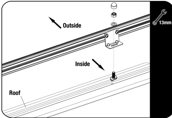
Place pre-assembled Side Profiles over the mounting points. Align feet with factory holes and secure the feet to the roof using M8 x 25 T-Bolts, M8 x 16 Flat Washers, and M8 Nyloc Nuts. You will need a friend to help. Fully tighten.
