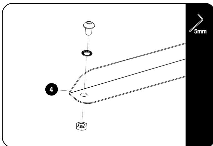
Loosely assemble the M8 x 12 Button Head Bolt, M8 Schnorr Washers and M8 Thin Nut both LH & RH Wind Deflectors (Item 4) as shown.
