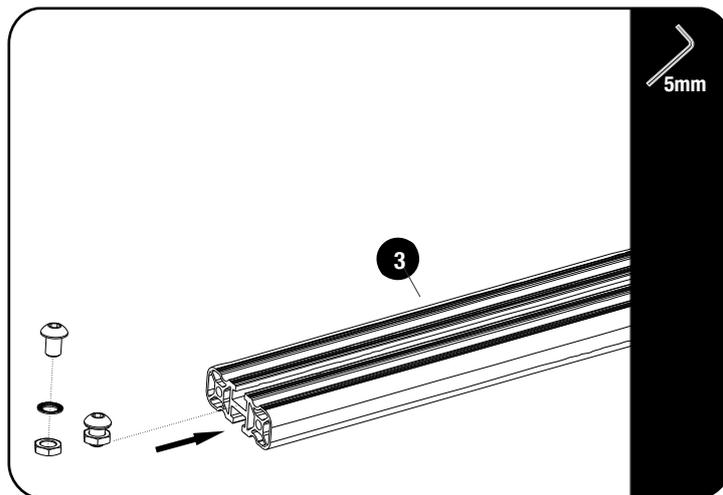
Insert two Button Head Bolts, M8 Half Nuts and M8 Schnorr Washers assemblies into the Narrow Slat as shown. Slide them to the center of the Narrow Slat (Item 3), making sure that the Schnorr Washer is above the T-Slot Channel.
