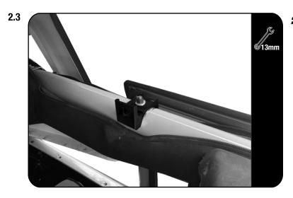
Loosly assemble the Roll Cage Bracket (Item 6) to the roll bar using M8 x 80 Hex Head Bolt, M8 x 25 x 3 Flat Washers, M8 x 19 x 3 Flat Washers and M8 Nyloc Nuts (Items 14, 15, 16 & 17) as shown in FIG 1.1.
