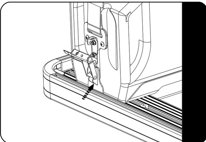
↻ Open the latch and hook it into the catch plate on the Jerry Can Holder Tray.
