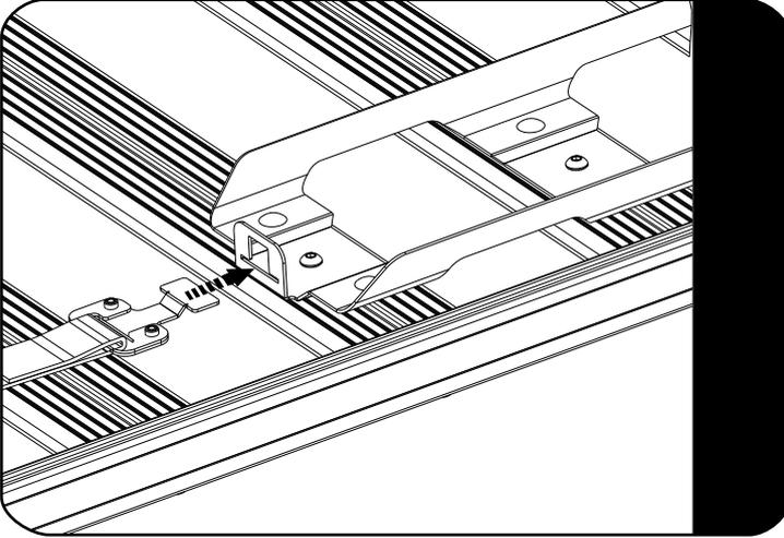
↻ Insert the rear hold plate on the Strap into the slot on the Jerry Can Holder Tray.
