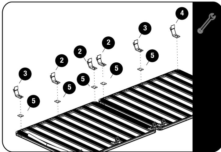
↻ Loosely assemble the Legs & Spacers (Item 2, 3, 4 & 5) as shown, slats indicated in 2.2 using M8 Flat Washers and M8 Nyloc Nuts included in the Leg sets.
